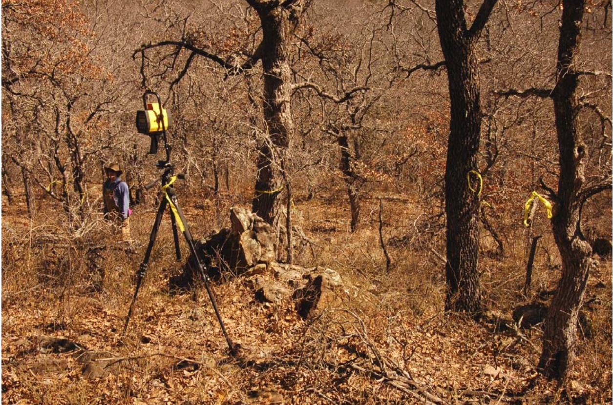
Figure 7. The Laser Atlanta Advantage Range Finder mounted on the tripod in the foreground was used along with a Trimble GeoXM GPS to map all trees to submeter accuracy. This mapping will facilitate future studies of vegetation change at Ft. Wolters. A portion of Plot B is illustrated in the photograph.
